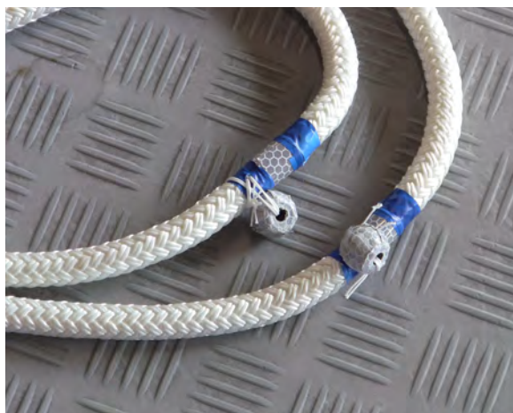
Figure 4: The reflective marker sewn on to the seine rope.
