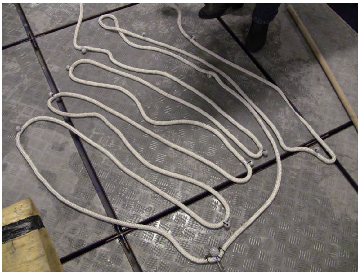
Figure 15: The combination rope laid out on the platform of the flume tank. Showing the very small bending stiffness
